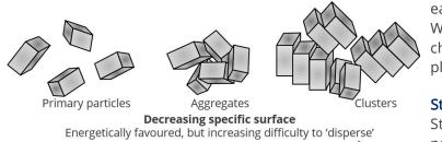
During the grinding process, these clusters can be broken down to the level of primary particles. The grinding process in the liquid phase consists of three processes:
